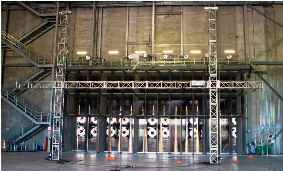
Figure 1: The horizontal gantry located near the front of the 55-foot turntable in the test chamber.
