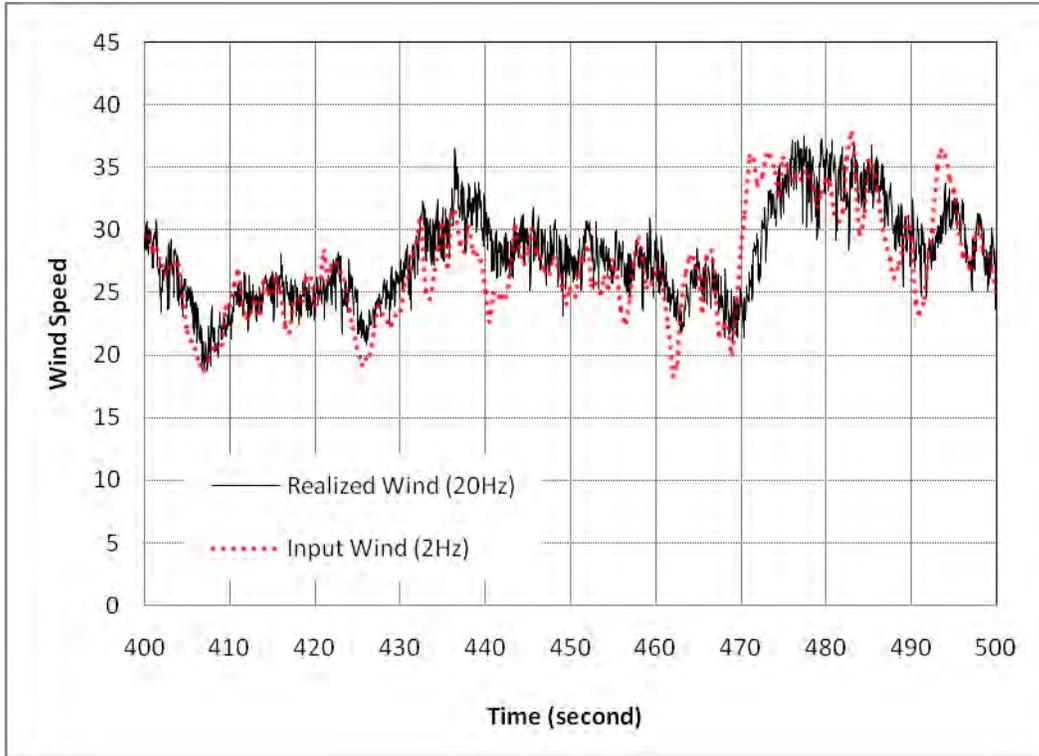
Figure 11: Comparison of input wind speed time history shown in Figure 7 with wind speed time history measured in the IBHS test facility using the Cobra Probe for the corresponding TTU record segment.
