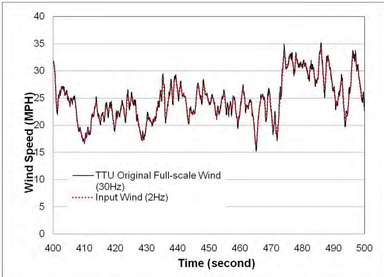
Figure 7: Comparison of TTU field measurements of wind speeds with the target 2-Hz record used as input control for fan speeds.
