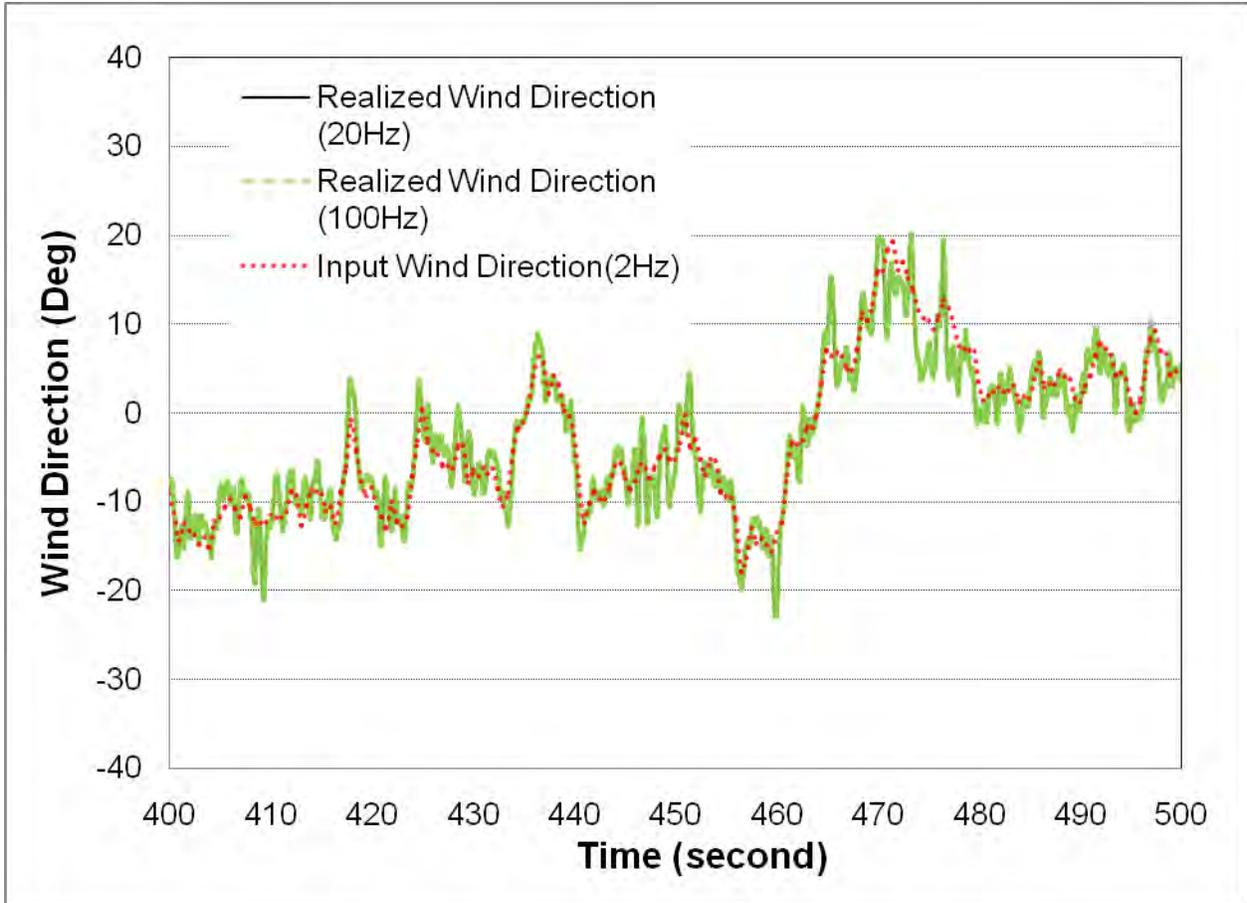
Figure 10: Comparison of input wind direction time history shown in Figure 8 with wind direction time history measured in the IBHS test facility for the corresponding TTU record segment.
