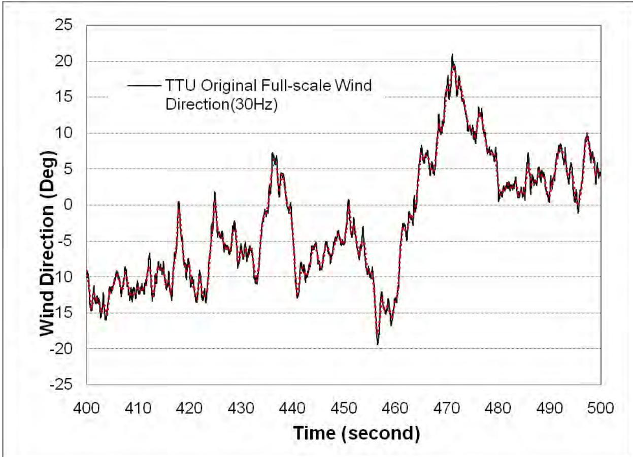
Figure 8: Comparison of TTU field measurements of wind direction with the target 2-Hz record used as input control for vane action.
