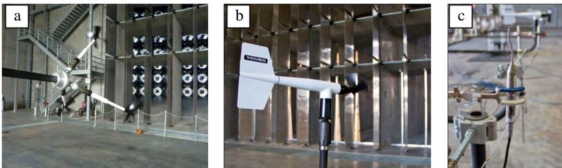
Figure 2: Flow measurement sensors: a) modified Gill UVW anemometer; b) R.M. Young wind monitor anemometer; and, c) Cobra probe on horizontal gantry.
