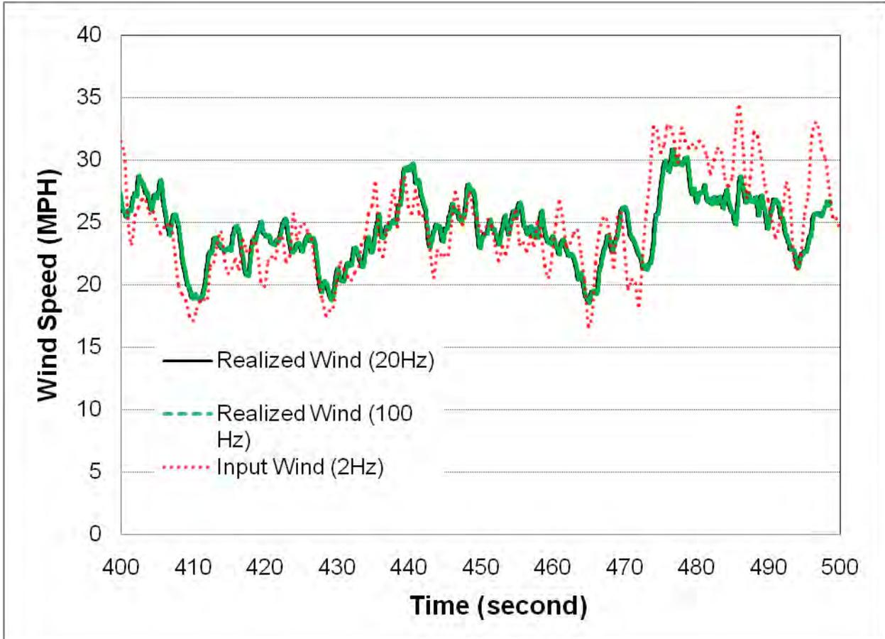
Figure 9: Comparison of input wind speed time history shown in Figure 7 with wind speed time history measured in the IBHS test facility for the corresponding TTU record segment.
