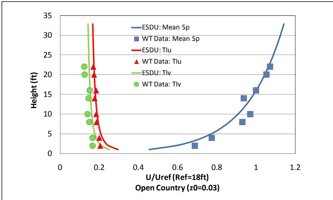
Figure 6: Mean wind speed profile and turbulence intensities for open country.
