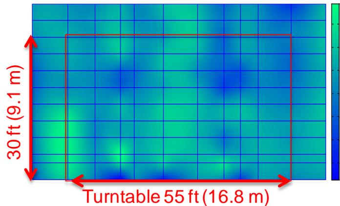
Figure 3: Uniform wind flow in the test chamber; changes in color show slight variations in mean wind speed.
