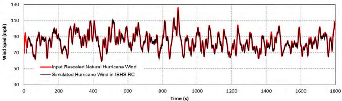
Figure 5: Comparison of simulated winds and input rescaled natural hurricane winds.
