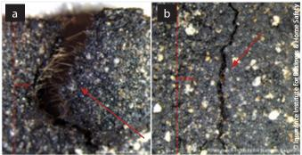
Figure 3a: Example of a tear visible at the edge of a shingle from the underside.
