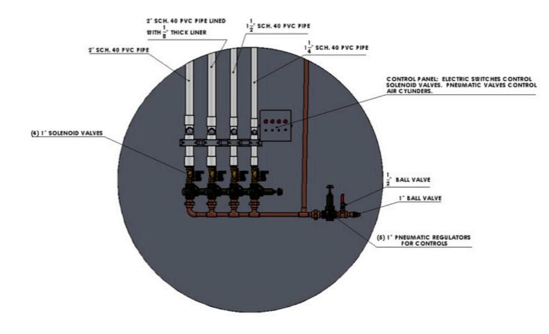
Figure A3: The control system is operated at ground level, where compressed air is regulated and valves opened to lift the appropriate size steel ball.
