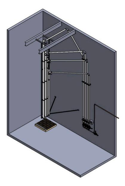
Figure A1: Overall diagram of the IBHS constructed UL 2218 test apparatus, shown mounted on the wall and ceiling.
