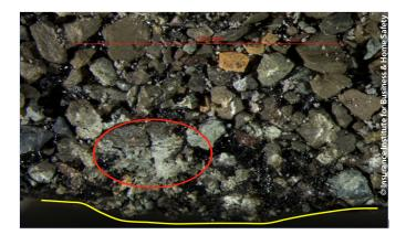
Figure 2: Common marks observed during UL 2218 tests included crushed granules (red circle) and flattening of the shingle edge (yellow trace). Image is magnified at 7.5x.
