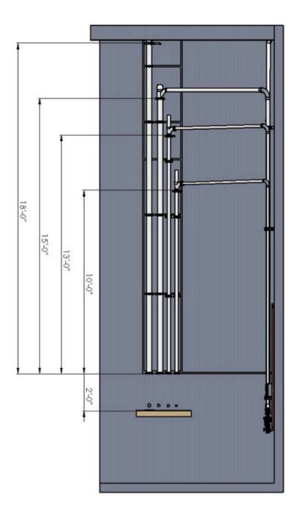
Figure A2: Drop tube dimensions.
