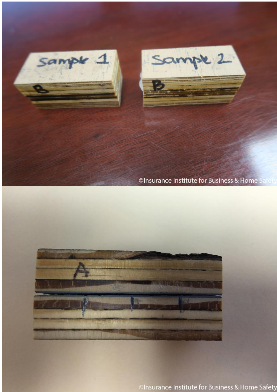
Figure 5. Prepared samples (top) with sanded edges (B side shown), and sample (bottom) divided into four sections (A side shown) for measuring paint film thickness.
