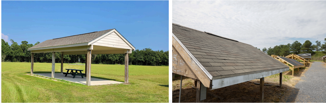
Figure 1. Collaborators can choose from two styles of specimen installation. On the left, the picnic hut style installation on a post system approximately 8 ft above ground level with a concrete pad underneath which is suitable to place picnic tables underneath. On the right, the traditional hut style installation on a post system approximately 4 ft above ground level.
