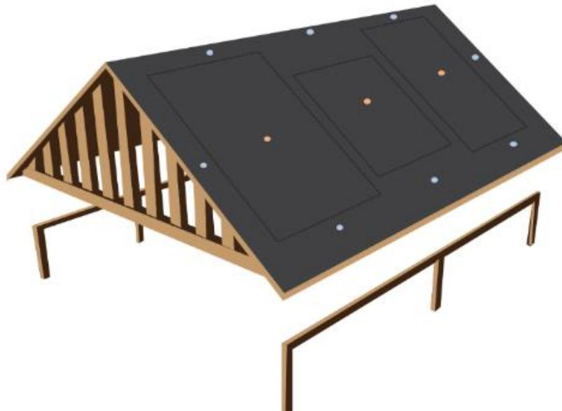
**Figure 1-1.** Diagram of a roof specimen showing temperature probe measurement locations. Note that for specimens at the Madison, Wisconsin, and Amelia, Ohio, sites, temperature probes are located on the center panel of each roof face only.
