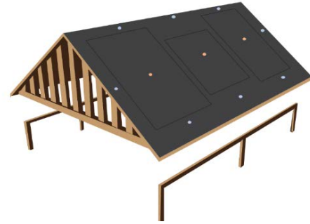
Figure 1-1. Diagram of a roof specimen showing temperature probe measurement locations. Note that for specimens at the Madison (Wisconsin) and Amelia (Ohio) sites, temperature probes are located on the center panel of each roof face only.
