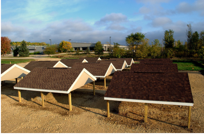
Figure 2-6. Photograph of the roof aging farm at American Family Insurance in Madison, Wisconsin.
