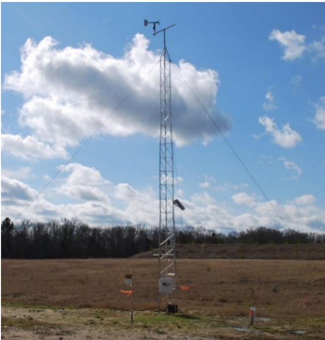
Figure 2-5. Photograph of the surface weather observing station at the IBHS Research Center. Photo was taken shortly after installation in 2011, before the roof aging farm installation began.
