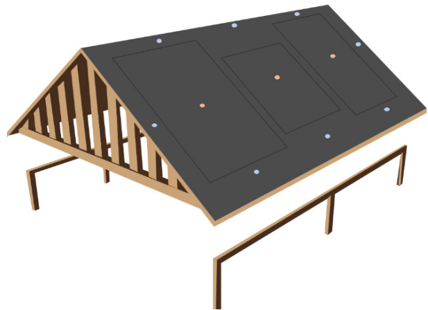
Figure 2-1. Example of a roof aging farm specimen, with three test panels per face. Thermocouple probe locations are indicated in brown for the standard instrumentation setup. At each location indicated, there are two probes: one between roof cover layers, and one between the underlayment and roof deck. Probe locations shown in blue correspond to high-density instrumentation of the 20-year specimens at IBHS, where one thermocouple is located between roof cover layers.
