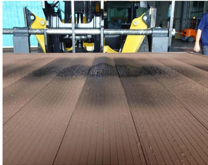
*Figure 2. Deck assembly with Type 1 walking surface and SYP after the test*
