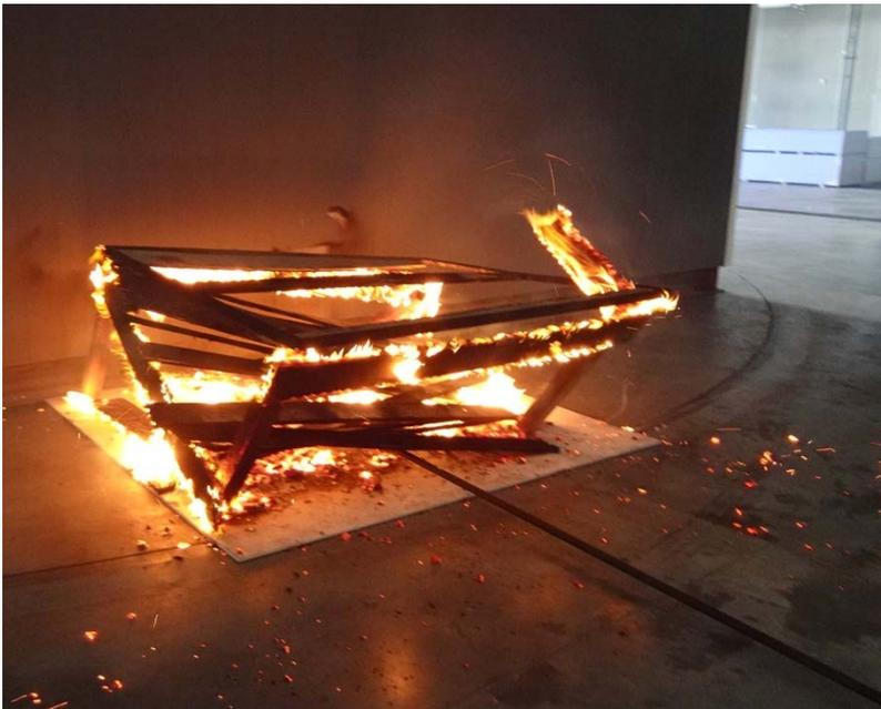
*Figure 3. Deck assembly with Type 2 walking surface and SYP at the last stages of the test*
