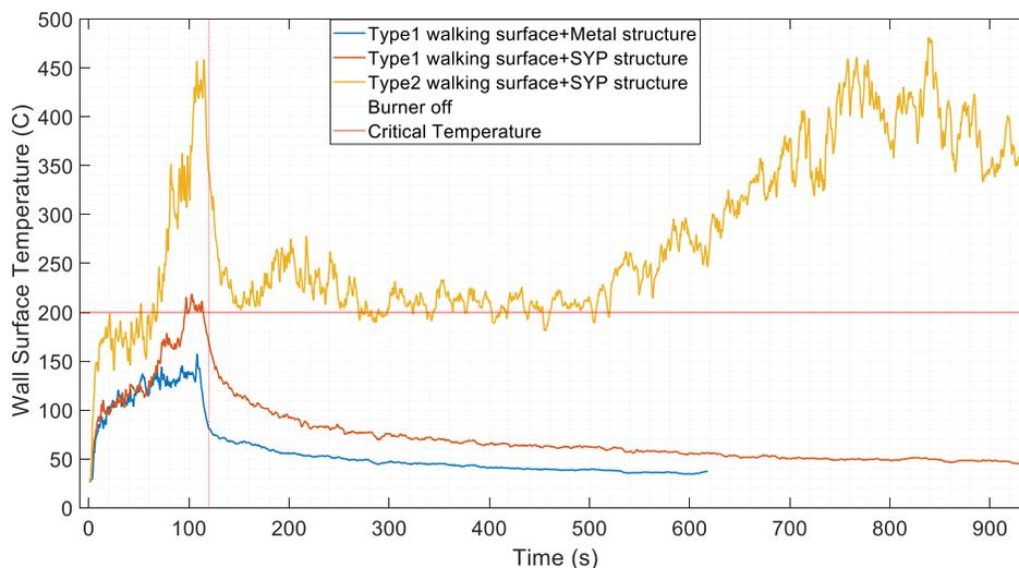
Figure 1. Wall surface temperature over time for the deck assemblies evaluated in this series of experiments. 200°C was selected as the critical, not-to-exceed, wall surface temperature.
