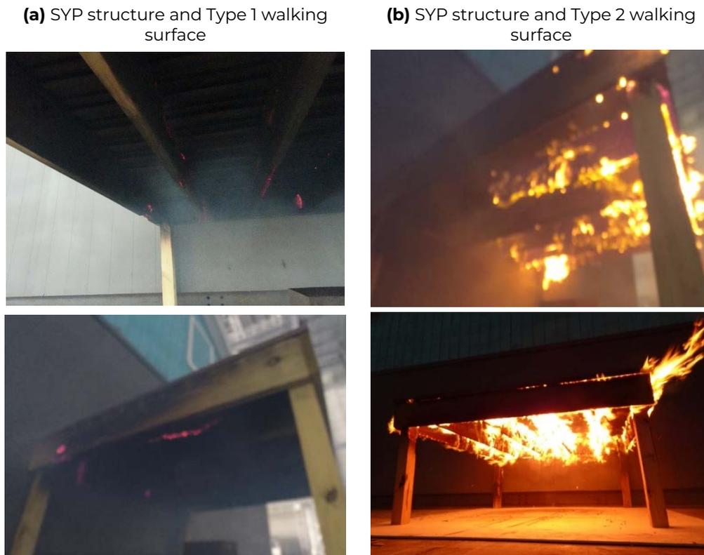
*Figure 4. Comparison of Type 1 (a) and Type 2 (b) walking surfaces installed over SYP substructure*
