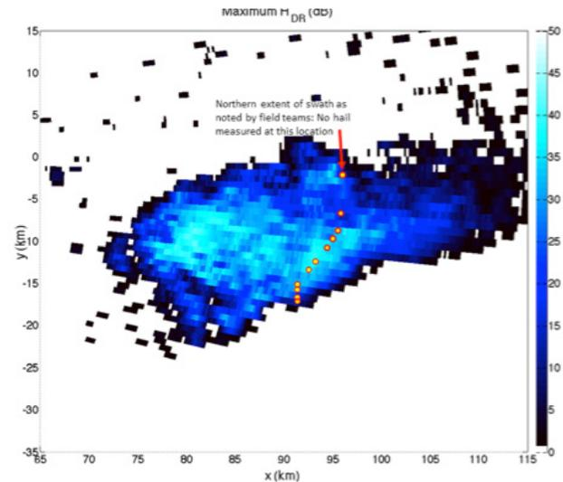
Figure 4: Experimental KFDR polarimetric HDR based hail swath from 7 May 2014 near Waurika, Oklahoma. The color-scale refers to the value of HDR (dB). Higher values are hypothesized to represent a larger confidence in the presence of hail. Field team observation locations are shown in yellow. Hailstones were not physically measured by the field teams at the northern-most observation location. Data are courtesy of Dr. Matthew Kumjian, Penn State University.
