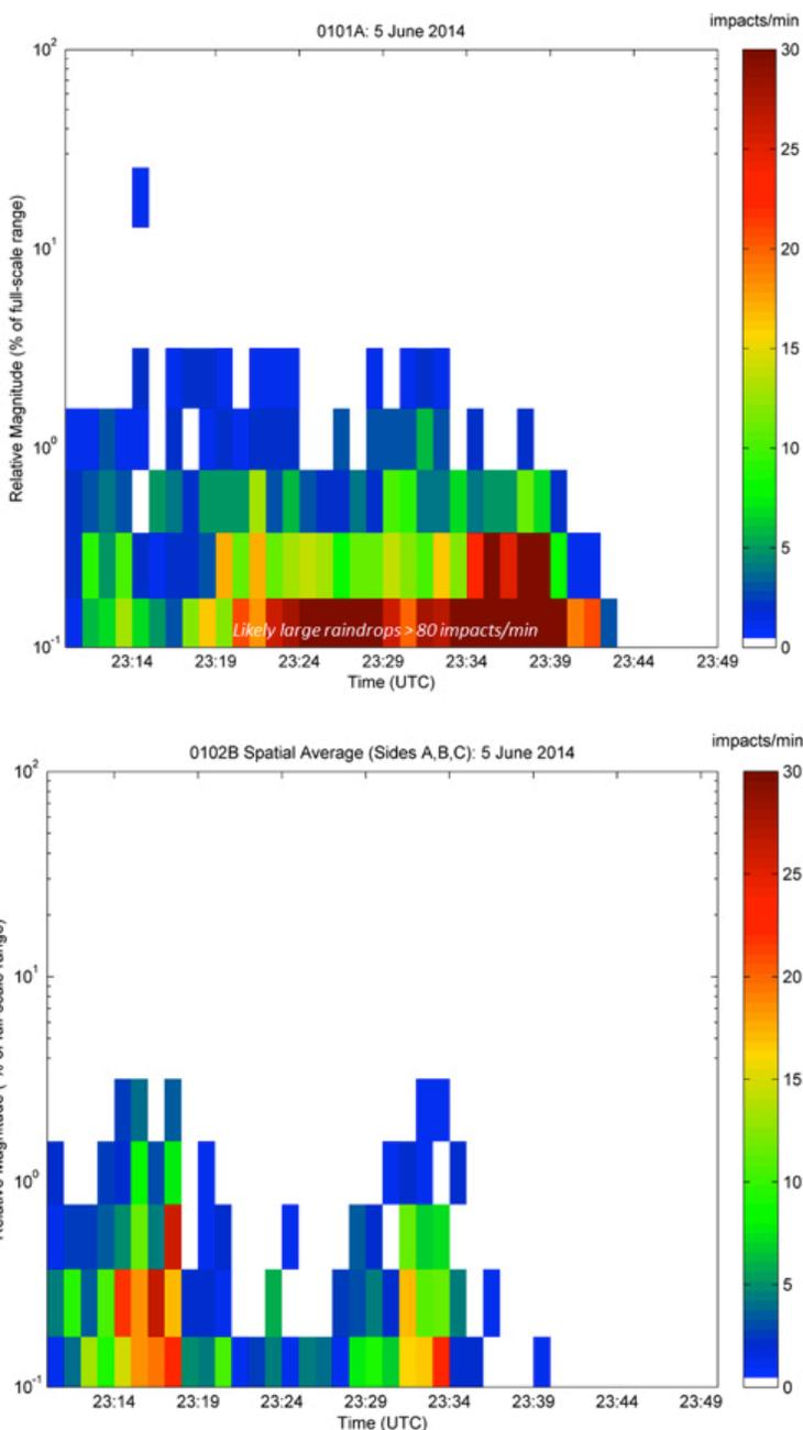
Figure 5: Impact concentrations per minute observed by probe 0101A (top) and 0102B (bottom) on 5 June 2014. The y-axis represents the relative-size of hail and/or large rain drops.
