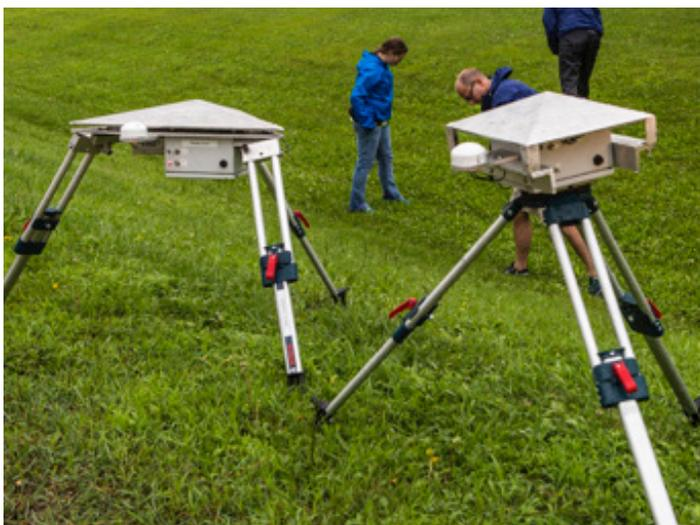
Figure 1: Photograph of the two prototype hail impact disdrometers (0102B-left, 0101A-right) deployed during the 2014 field phase.
