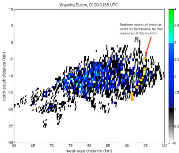
Figure 3: Experimental polarimetric radar-based hail swath from 7 May 2014 near Waurika, Oklahoma. The color scale represents the number of occurrences where the horizontal reflectivity exceeded 50 dBZ and the ZDR was 0 or less. Field team hail observation locations are shown in yellow. Hailstones were not physically measured by the field teams at the northern-most observation location. Data are courtesy of Dr. Matthew Kumjian, Penn State University.
