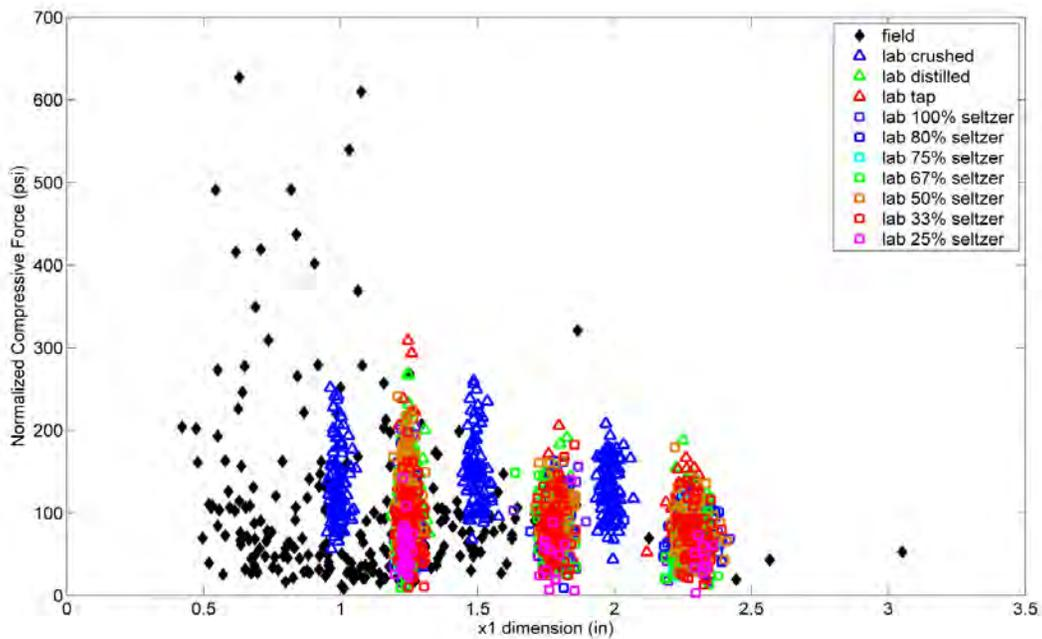
Figure 6: Comparison of field and laboratory compressive force values as a function of the measured  $x_1$  dimension.
