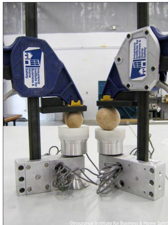
Figure 1. Two IBHS prototype field compressive force measurement devices.
