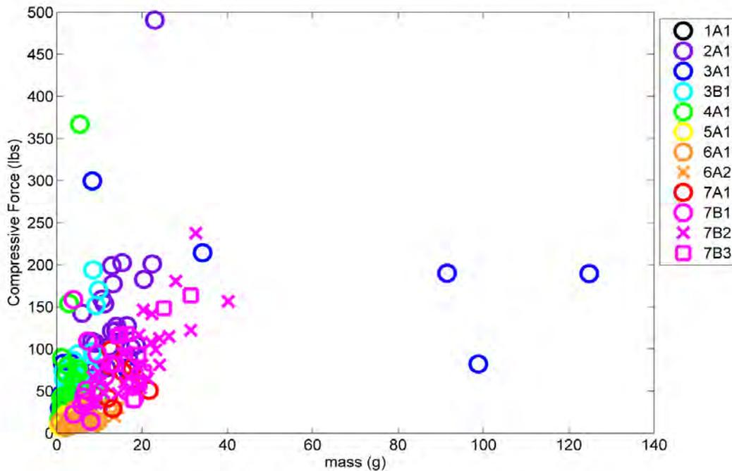
**Figure 5. Measured compressive force as a function of the measured mass. Each color circle represents data points from a single storm, while additional symbols of the same color indicate more than one deployment on a single storm.**
