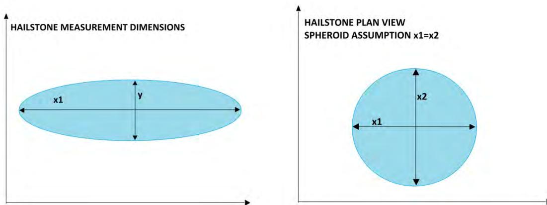
Figure 2. Diagram of the measured dimensions of hailstones. Each stone was assumed to be a spheroid in shape with dimensions  $x_1$  and  $x_2$  equal. Only dimensions  $x_1$  and  $y$  were measured in the field.
