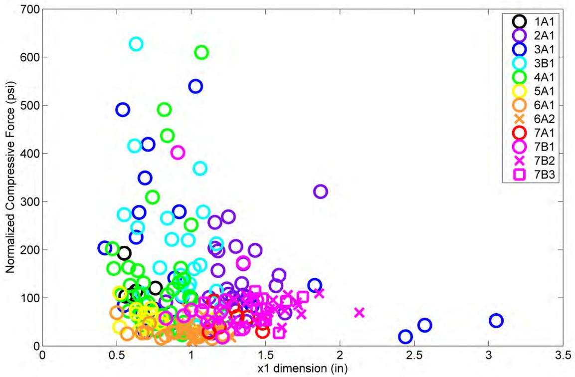
Figure 4. Normalized compressive force as a function of the measured  $x_1$  dimension. Each color circle represents data points from a single storm, while additional symbols of the same color indicate more than one deployment on a single storm.
