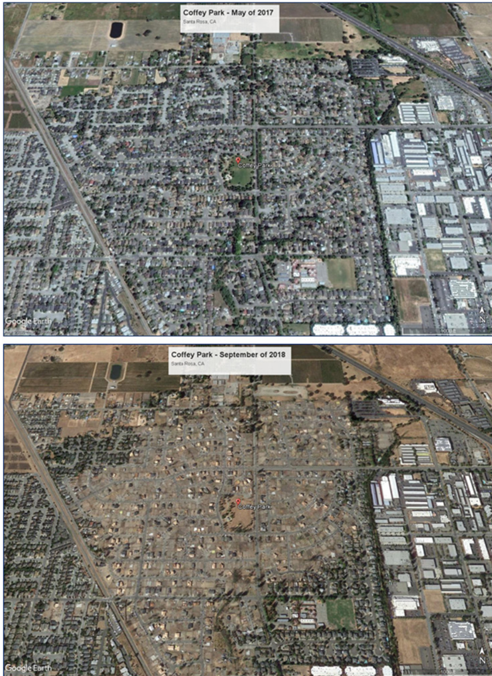
Figure 4: Aerial imagery of the Coffey Park neighborhood in Santa Rosa, California, before the Tubbs fire in May 2017 (top), and after the fire (bottom). The average spacing between adjacent walls of homes was approximately 10 ft. Imagery courtesy of Google Earth.
