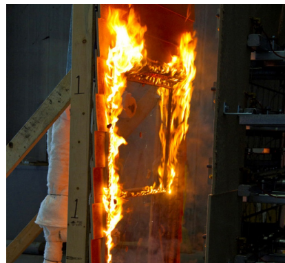
Radiant heat. The radiant heat caused the glass to break and the window frame to ignite.
