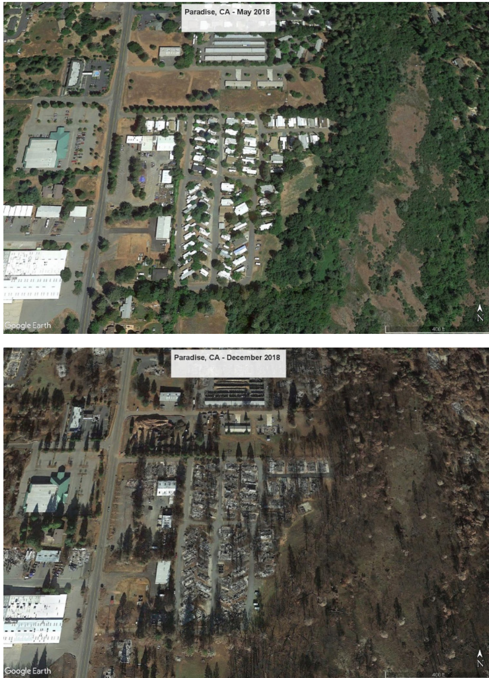
Figure 5: Aerial imagery of a manufactured-home community in Paradise, California, (top) in May 2018 prior to the Camp Fire, and after the fire (bottom). The average distance between structures was approximately 18 ft. Aerial imagery courtesy of Google Earth.
