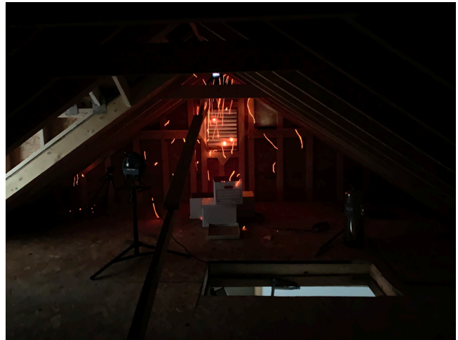
Figure 7: Time exposure photograph tracing embers entering the gable-end vent and a ridge vent on a test home at the IBHS Research Center.
