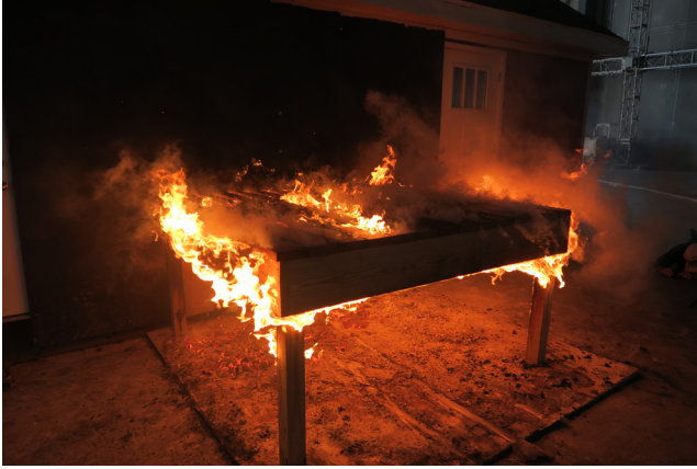
Figure 6: Images of deck testing at the IBHS Research Center show how (left) an intense fire can develop under a deck and (right) can spread toward a home's wall.
