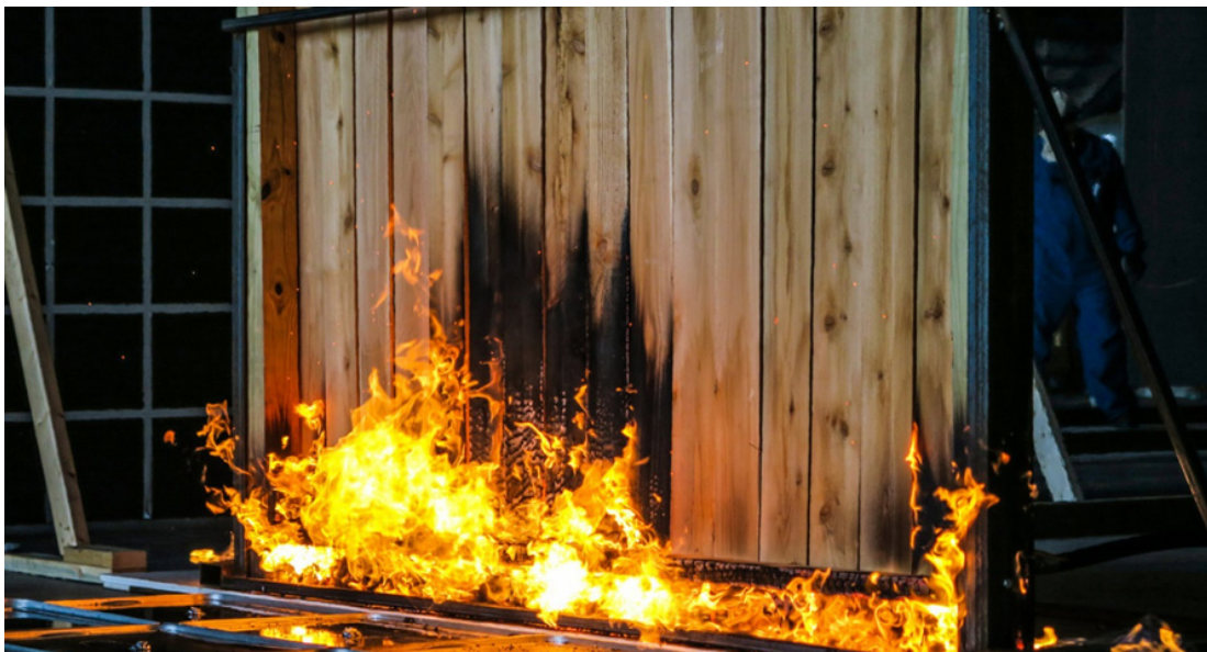
Figure 12. Top: Fence with evidence of burning that was knocked down. Bottom: a similar combustible wood fence during testing at the IBHS Research Center.
