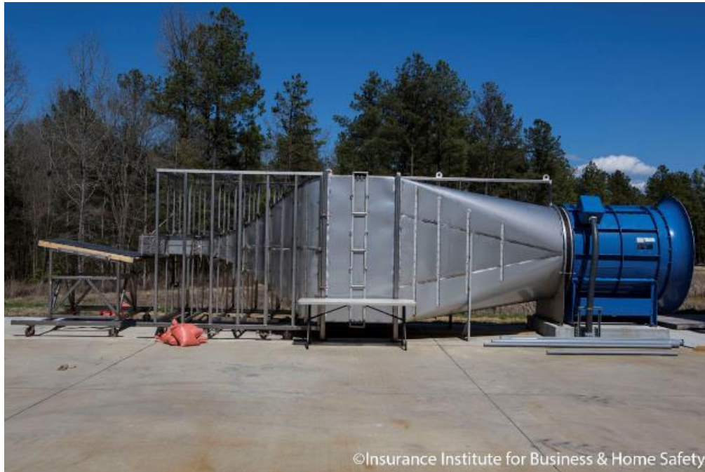
Figure 2. IBHS Component Materials Evaluation Tester (COMET). This is a single-fan test apparatus that can test the wind performance of materials up to 170 mph. Panels are tested at 2:12 pitch and exposed to a steady speed wind for two-hour increments if they pass 60 mph and 90 mph 10-minute-long tests. Tests were performed when the temperature was 75°F +/- 10°.
