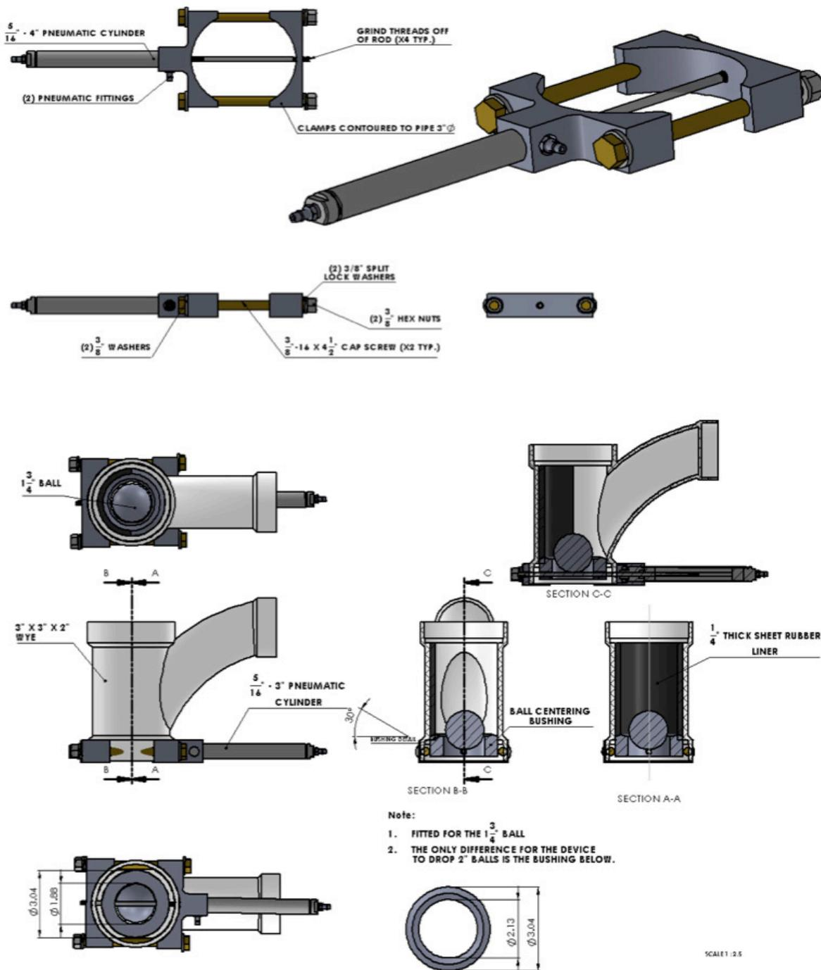
Figure A4: Drawings illustrate the entry of the steel ball into the drop tube, where it is secured in place until the operator presses the trigger button. The pneumatic cylinder then releases, and the ball is dropped.
