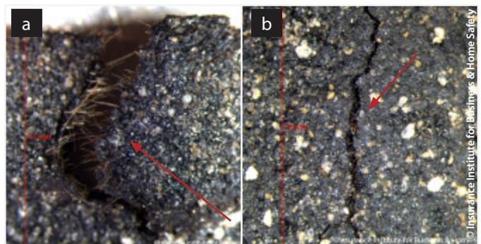
Figure 3a: Example of a tear visible at the edge of a shingle from the underside.
