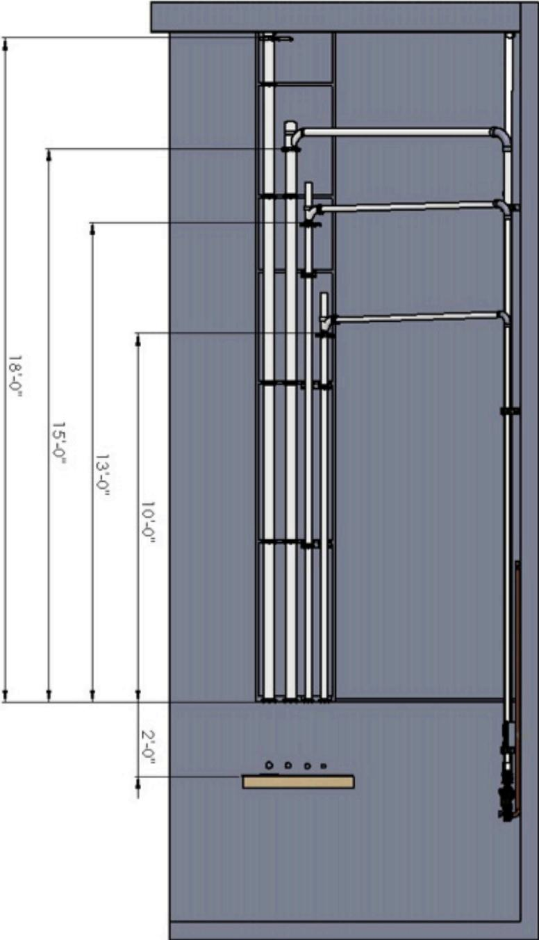
Figure A2: Drop tube dimensions.
