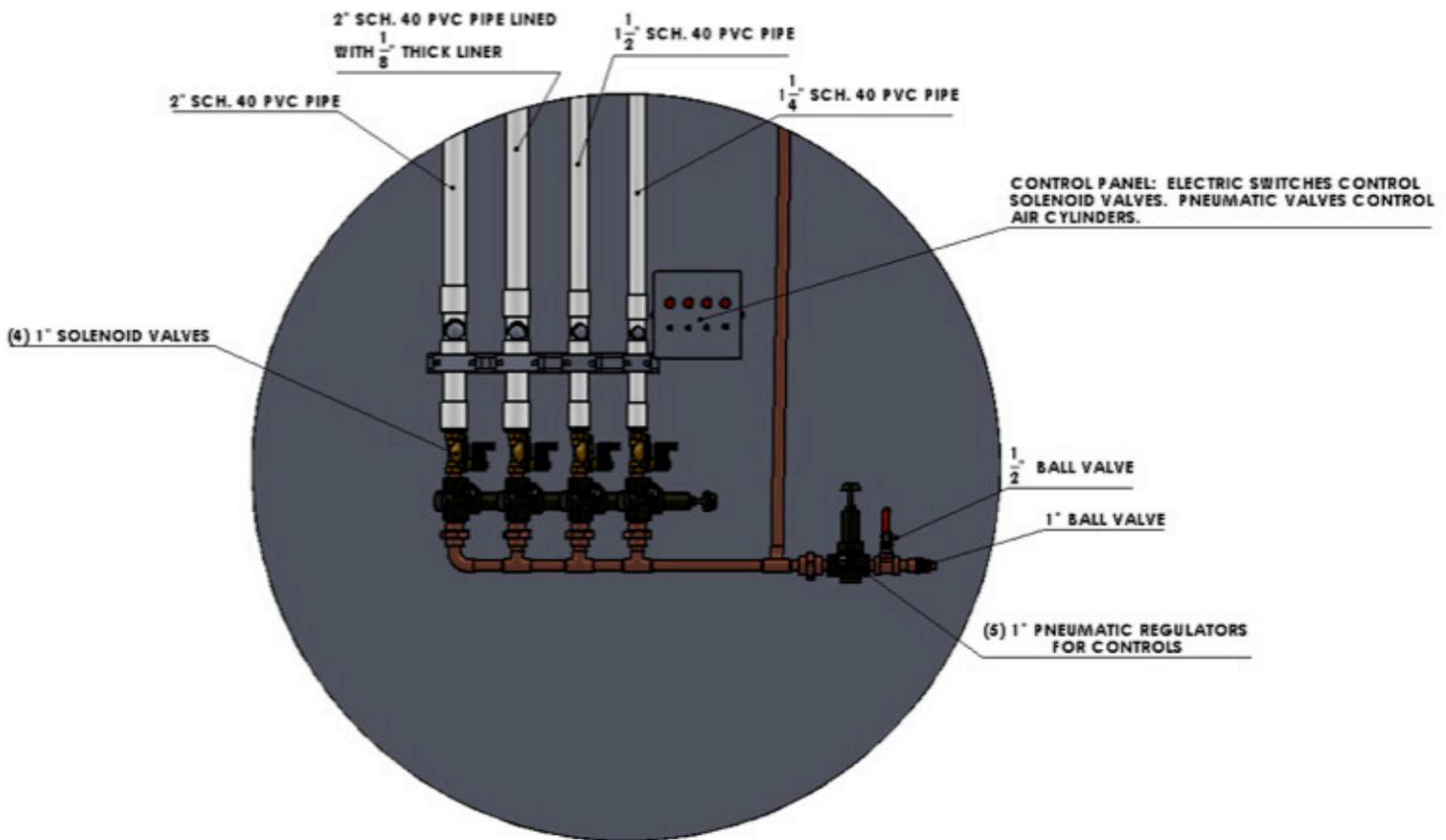
Figure A3: The control system is operated at ground level, where compressed air is regulated and valves opened to lift the appropriate size steel ball.
