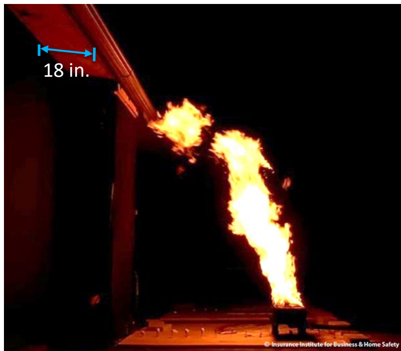
Figure 10. Direct flame contact to the soffit and gutter during an ambient wind condition (zero wind speed) test with the fire exposure positioned 5 ft from the building.
