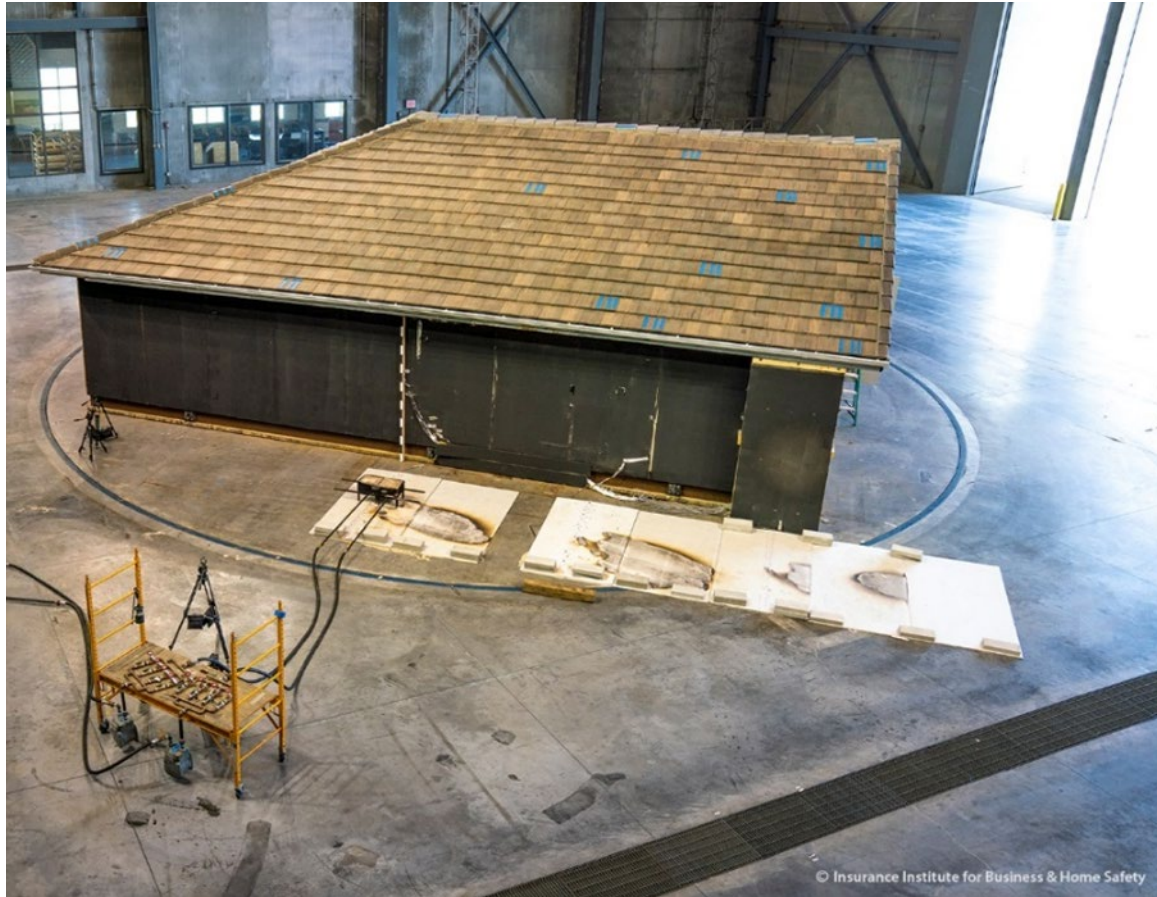
Figure 1. Overview of experimental setup with 30-ft x 40-ft building. This image shows a 45-degree test with the building rotated so the corner is closest to the fans.
