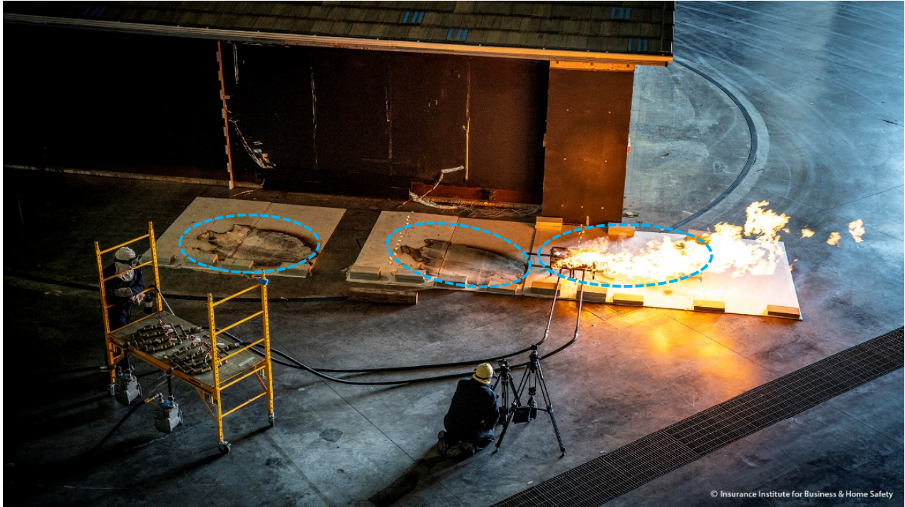
Figure 6. Burner and instrumented wall at the E-R location, 5-ft separation from building, idle wind speed. Dashed-blue circles indicate areas from previous tests where flame scorched the ground.
