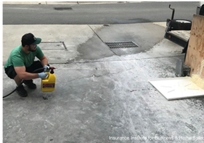
Figure 1: Application of a gel product to the T1-11 plywood samples.
