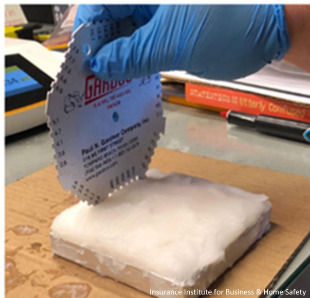
Figure 2: Measuring the wet film thickness of a gel product.
