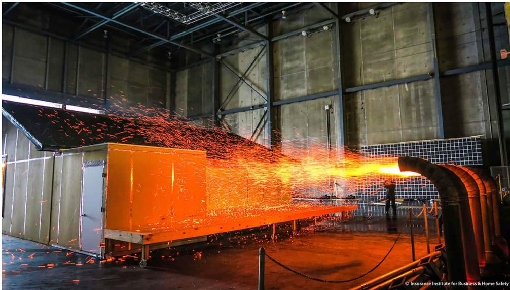
Figure 10. Testing deck vulnerability to embers at the IBHS Research Center. IBHS and others have [conducted extensive testing](#) regarding the vulnerability of decks<sup>53</sup> and fences.<sup>54</sup>
