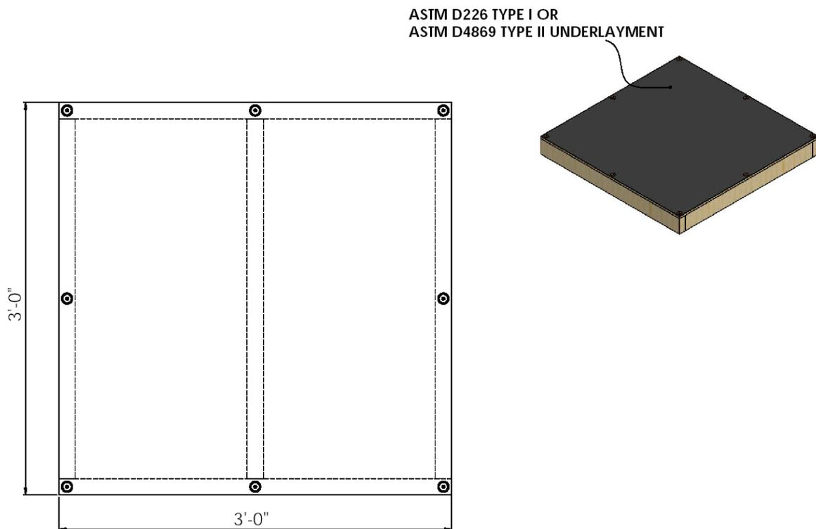
**Figure 5.3.1-1.** The underlayment is applied to the test deck with button-cap nails driven straight and flush and spaced along the outer frame at each corner and the center of each edge.
