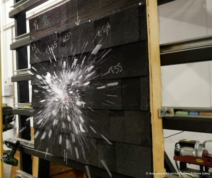
**Figure 3.16.2-1.** Hard shatter Impact Mode ice spheres will break into many fragments upon impact with the test sample assembly.
