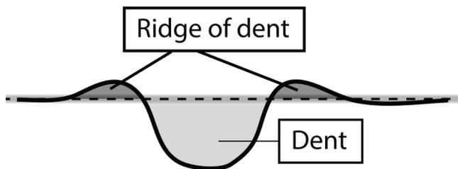
**Figure 3.18-1.** The negative local deformation caused by a dent and the positive local deformation at the ridge of dent.
