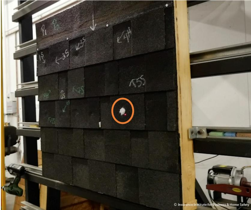
**Figure 3.16.1-2.** Soft Impact Mode ice spheres will leave a slushy residue (larger than 18 mm for class 1.5 impacts and larger than 24 mm for class 2.0 impacts) on the test sample assembly upon impact.
