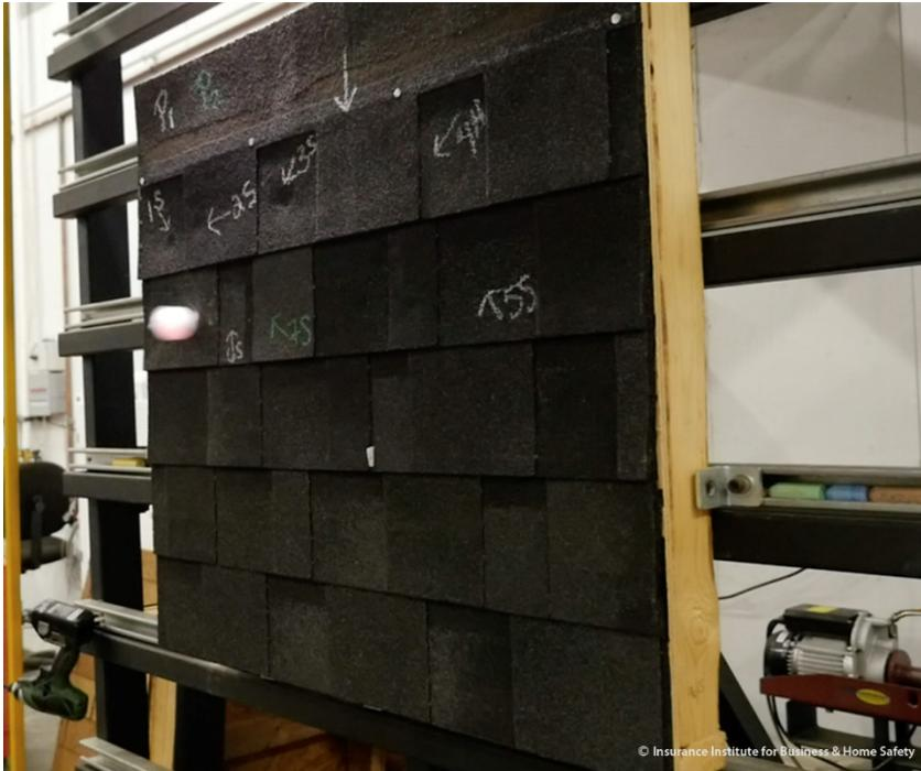
**Figure 3.16.3-1.** Hard bounce Impact Mode ice spheres will not break upon impact with the test sample assembly and will bounce back as a single piece.
