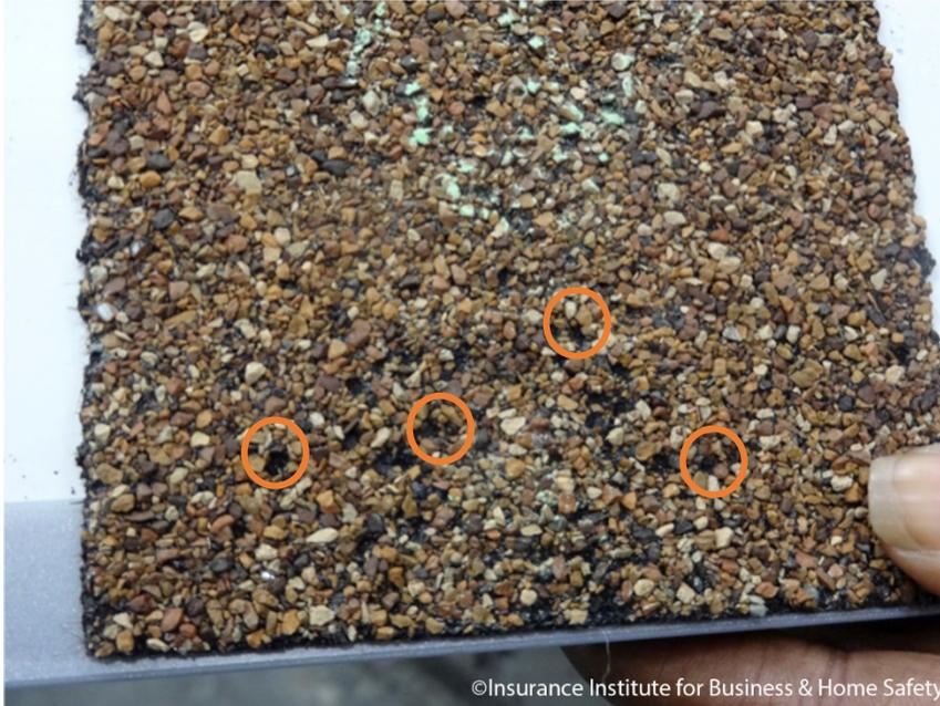
**Figure 3.18.2.2-1.** Example photograph of individual granule loss.
