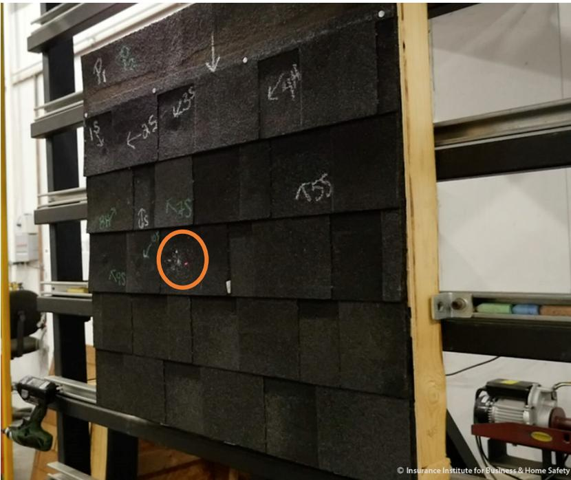
**Figure 3.16.2-2.** Hard shatter Impact Mode ice spheres may or may not leave a slushy residue (smaller than 18 mm for class 1.5 impacts and smaller than 24 mm for class 2.0 impacts) on the test assembly upon impact.
