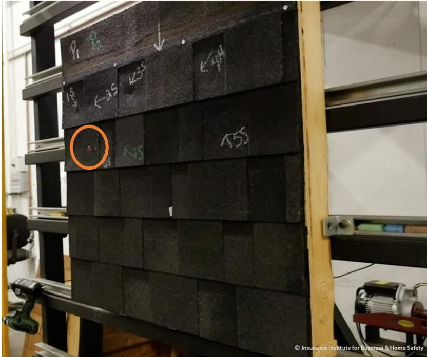
**Figure 3.16.3-2.** Hard bounce Impact Mode ice spheres will not leave a slushy residue on the test assembly upon impact.
