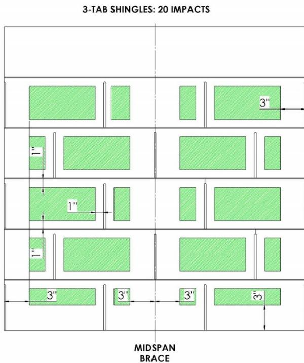
**Figure 8.5-1.** Impact location options for 3-tab shingles following the requirements of Table 8.5 and Section 8.5.1. (1 in. = 2.54 cm; 3 in. = 7.62 cm.)
