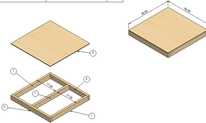
Figure 5.2.1-1. Assembly requirements for test decks.
