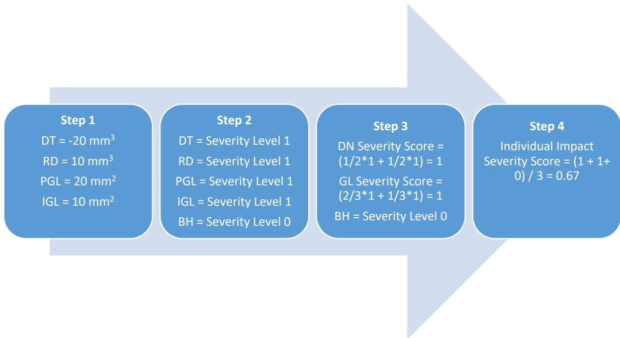
**Figure C9.7-1.** Example Individual Impact Severity Score.
