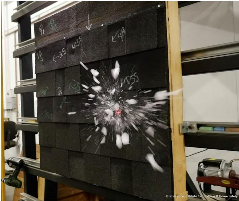
**Figure 3.16.1-1.** Soft Impact Mode ice spheres will break into many fragments upon impact with the test sample assembly.
