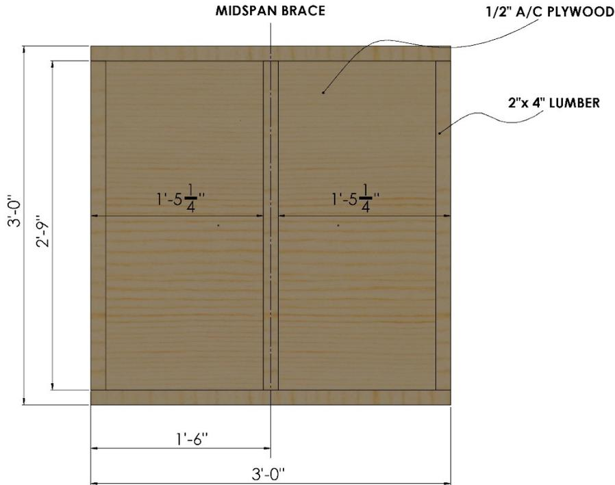
Figure 5.2.1-2. Bottom view of the test desk to illustrate the midspan support brace.
