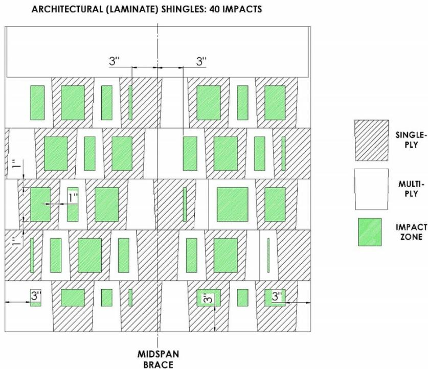
**Figure 8.5-2.** Impact location options for architectural shingles following the requirements of Table 8.5 and Section 8.5.1. (1 in. = 2.54 cm; 3 in. = 7.62 cm.)
